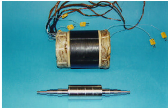
Figure 2. Permanent Magnet Rotor and Stator Details.
