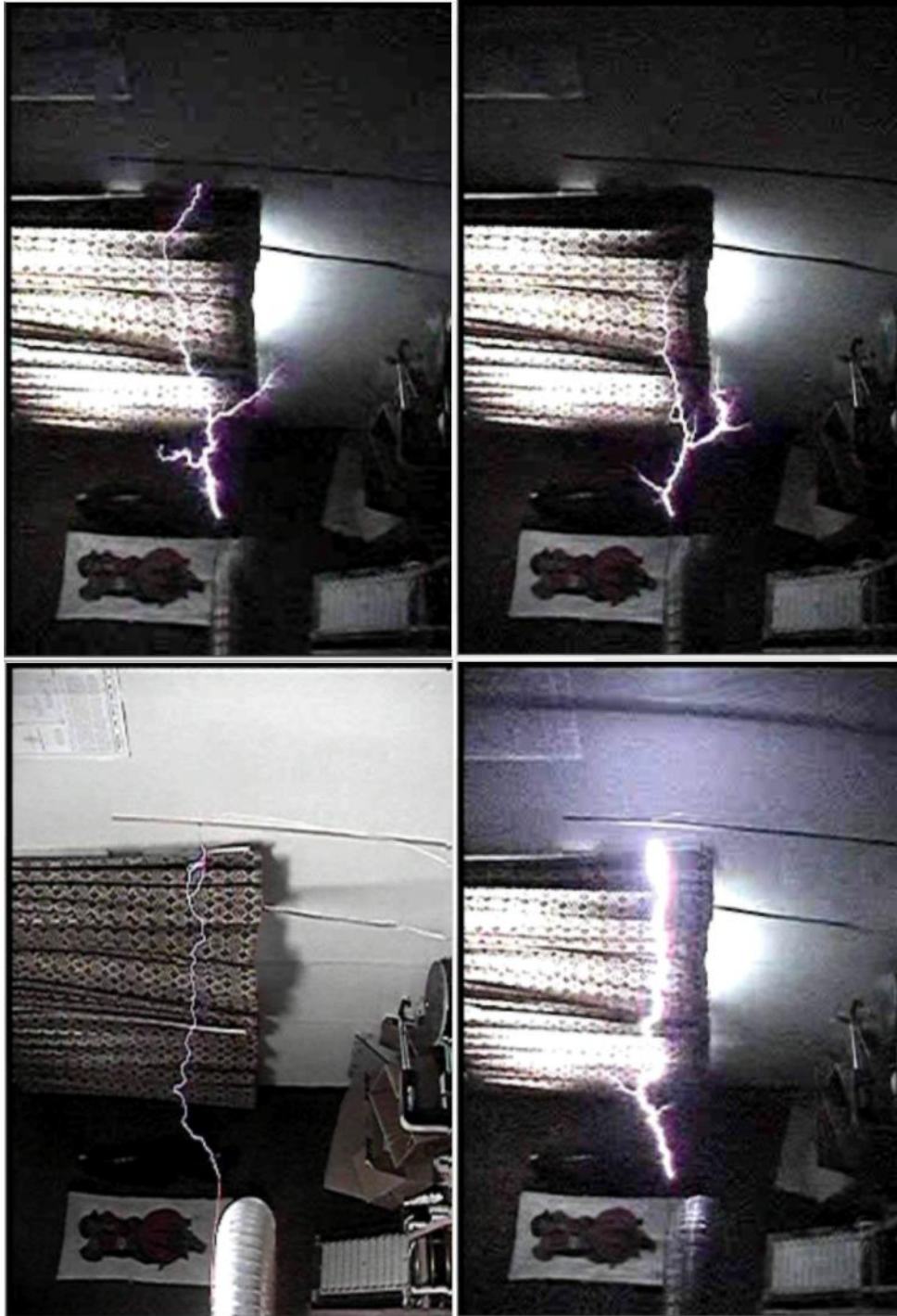
Figure 21. 30 inch arcs to ground at 183 watts.
