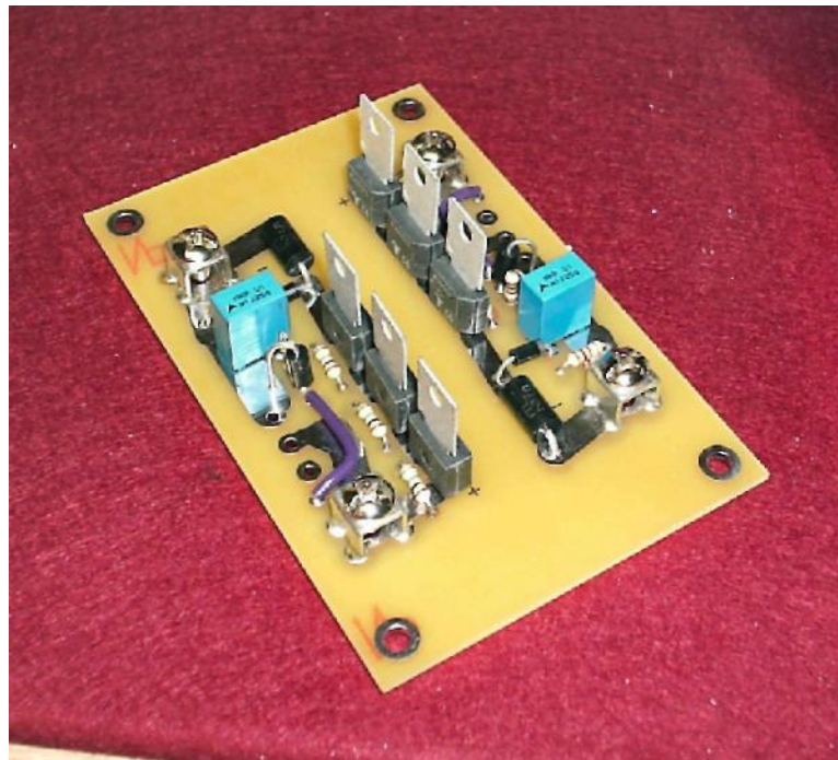
Figure 17. Actual SISG board less IGBTs.
