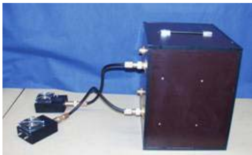
Figure 7 Synchronization of 4 RHL020M setup and measurement of the field at great distance
